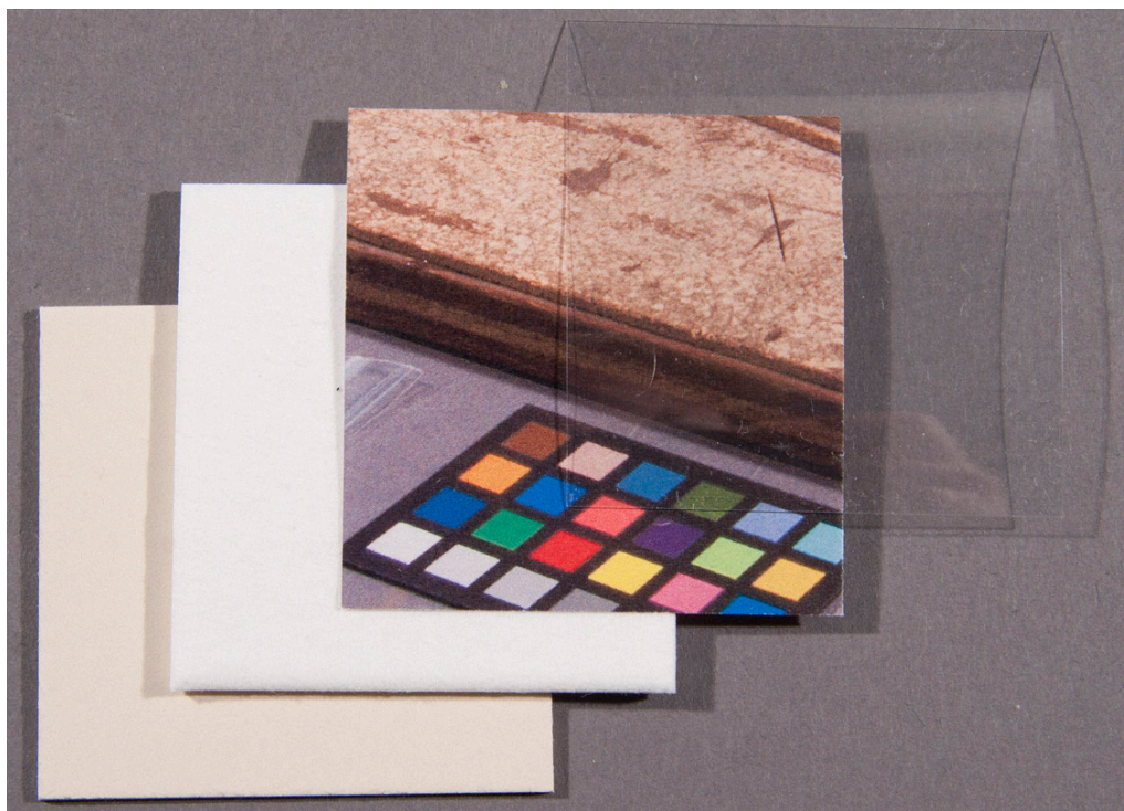
Figure 6: Dummy: Cardboard, blotting paper, colored paper, and domed Mylar®
