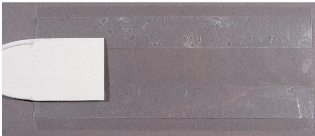
Figure 7: Mold: Mylar® strip adhered on silicone-coated carrier using double-sided pressure-sensitive tape
